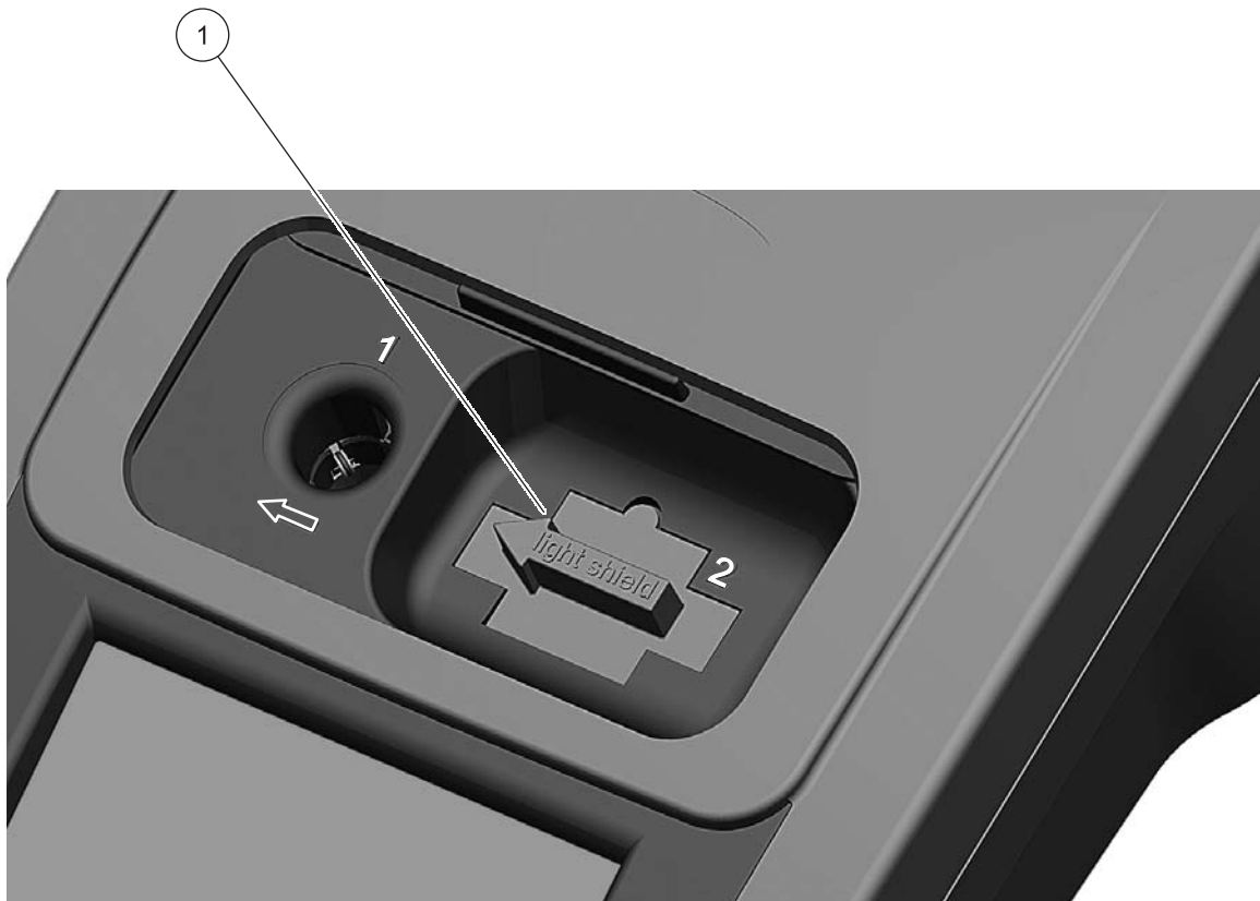
Figure 7 Light Shield in place
